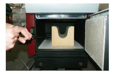
Each time before lightning up the boiler it is recommended to clean loading chamber. Ash needs to be removed through the nozzle. Use the tools supplied with the boiler.
